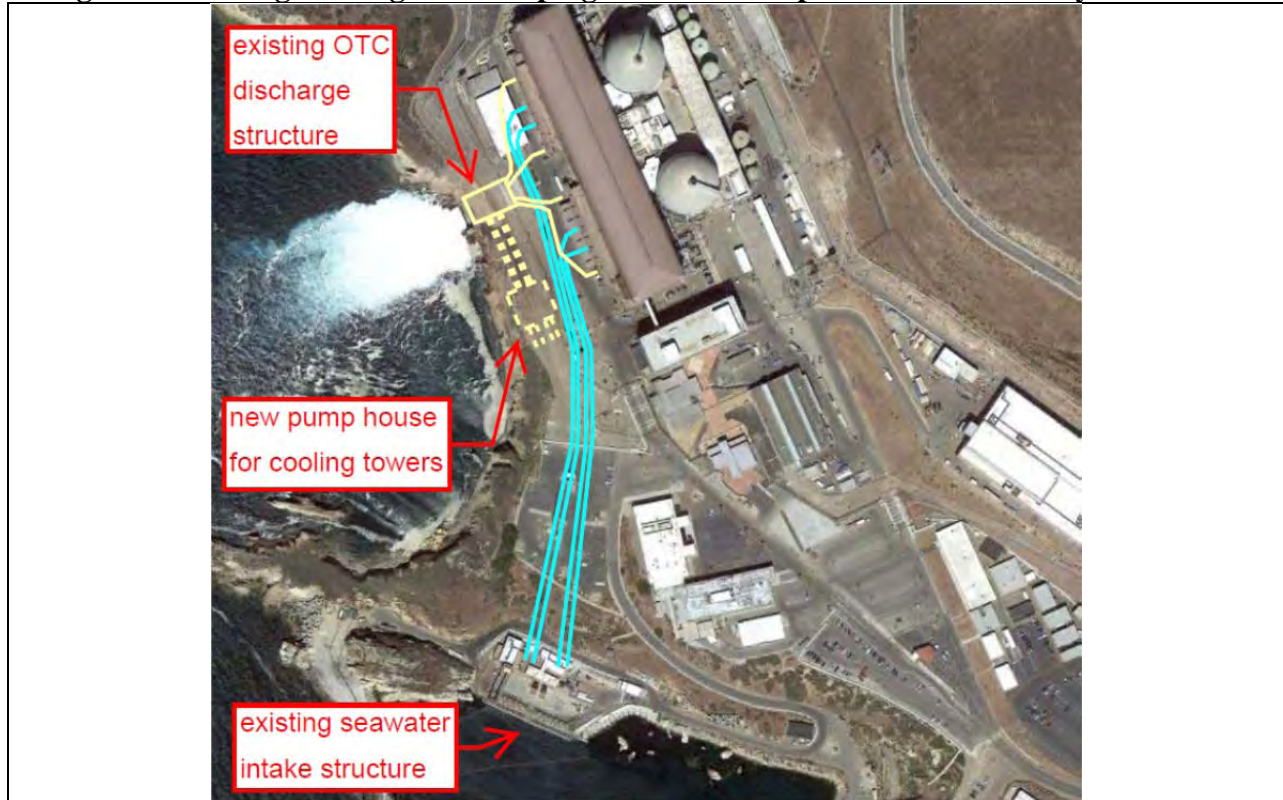
Figure 6. Existing Cooling Water Piping and New Pump House Identified by TetraTech
